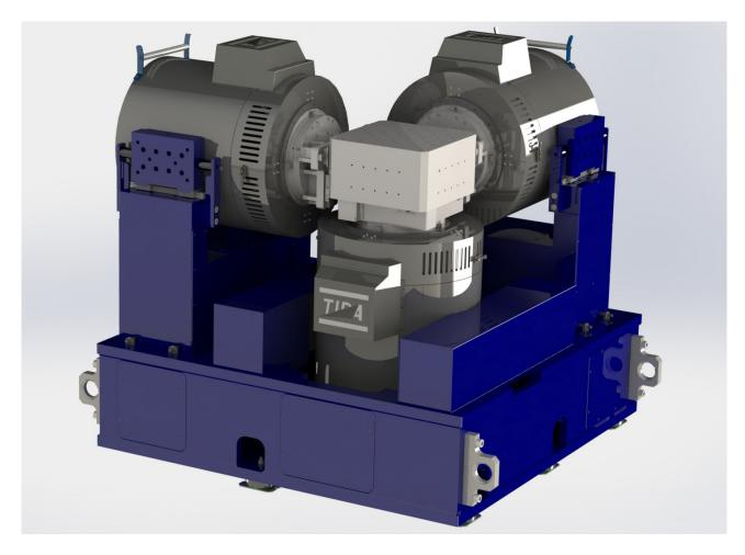
Our aim is to encourage our automotive customers' trust in our expertise with our new testing facilities. Our new 3-axis simultaneous testing machine meets the specifications according MIL standards, suitable for the automotive and aviation industries, and we can offer tests in a wide frequency range up to 2000 Hz.
